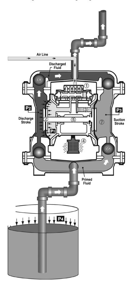
Air-Operated Double Diaphragm (AODD) pumps are powered by compressed air, nitrogen or natural gas.
