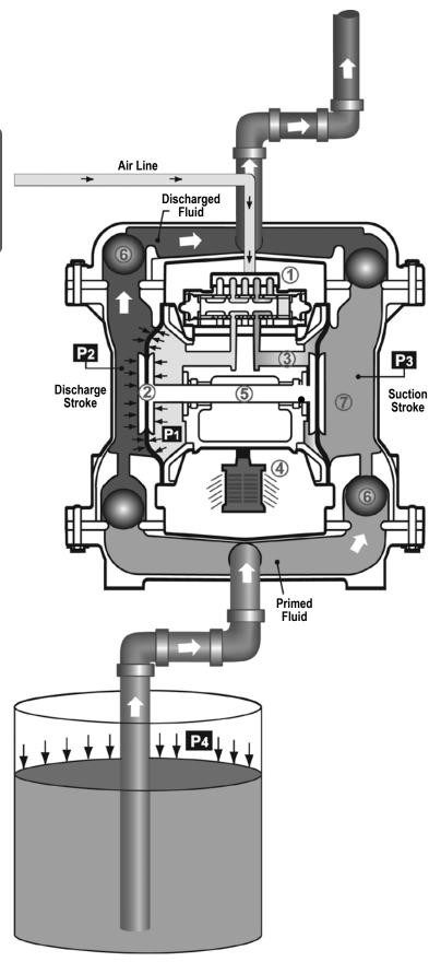
Air-Operated Double Diaphragm (AODD) pumps are powered by compressed air, nitrogen or natural gas.
