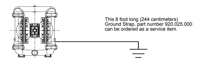
To reduce the risk of static electrical sparking, this pump must be grounded. Check the local electrical code for detailed grounding instruction and the type of equipment required, or in the absence of local codes, an industry or nationally recognized code having jurisdiction over specific installations.
