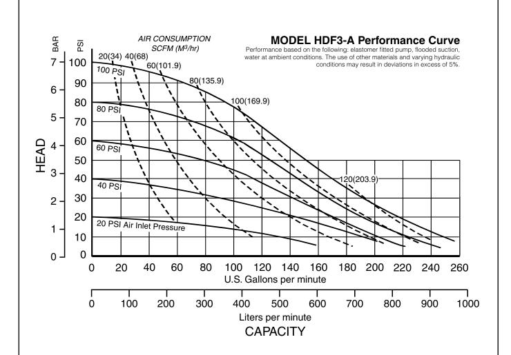
SANDPIPER® pumps are designed to be powered only by compressed air.
